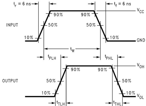
Figure 6. AC Waveforms
